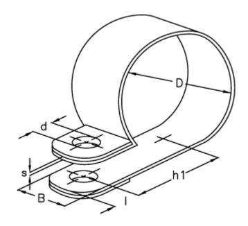
$\begin{array}{ll} d & = 10.5 \\ \text{Diameter D} = 63 \\ \text{h1} & = 46.0 \\ \text{I} & = 10.0 \\ \text{s} & = 1.2 \\ \text{Width B} & = 25 \\ \end{array}$
